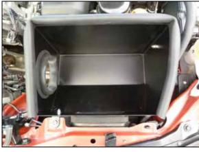
12. Set the heat shield into position on the core support and secure with the factory air box mounting bolts and to the previously install bracket with the hardware provided.
