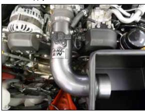
14. Install the tube through the heat shield. Rotate the tube down and install it into the silicone hose on the throttle body. Secure the tube with the provided hose clamp. NOTE: The tube is a tight fit through the opening, take care so as not to damage the edge trim.
