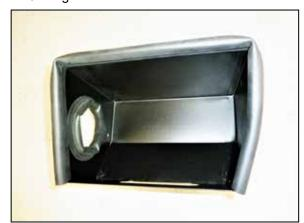
10. Install the 13" long section of edge trim into the hole of the heat shield as shown and then install the 27" long section of edge trim onto the top of the heat shield as shown.
