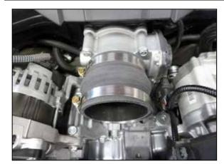
7. Install the provided silicone hose (08171) onto the throttle body and secure with the provided hose clamp.
