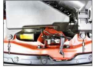
4. Remove the two bolts shown securing the resonator and air box to the core support. **NOTE:** These bolts will be reused in a later step.
