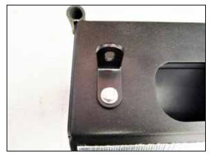
11. Install the provided "L" bracket (070066) onto the heat shield using the provided hardware.
