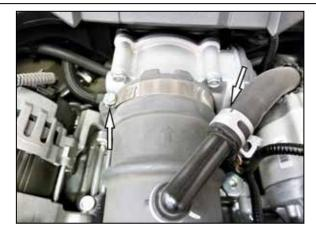
3. Release the spring clamp and then disconnect the crank case vent hose from the fitting. Loosen the hose clamp securing the intake hose to the throttle body.
