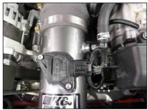
15. Connect the crank case vent to the fitting installed into the K&N intake tube as shown. Reconnect the mass air sensor electrical connection.
