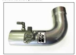
13. Remove the mass air sensor from the factory air filter housing and then install it into K&N intake tube using the provided hardware. Install the provided 90\* vent fitting into the K&N intake tube as shown. Apply the K&N decal as shown.
