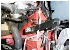
6. Install the provided heat shield mounting bracket (070026) onto the lower air box mount using the factory bolt.
