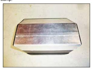
8. Install the provided heat shield insulation strips onto the bottom of the heat shield as shown. Some trimming of the insulation strips excess will be necessary.
