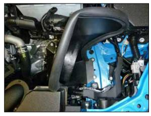
13. Install the heat shield assembly into the vehicle and secure with the provided hardware.
