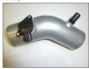
16. Remove the mass air sensor from the factory housing and install it into the K&N® intake tube and secure with the provided hardware. Install the vent fitting into the K&N® intake tube as shown.
