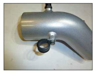
17. Install the provided cushion clamp onto the K&N® intake tube using the provided hardware.
