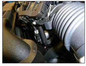
4. Unhook the solenoid bracket from the intake tube.
