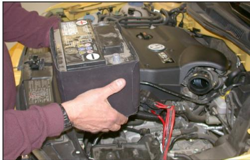
19. Remove the battery as shown.
