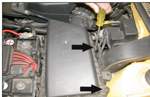
6. Remove the air cleaner cover screws as shown.
