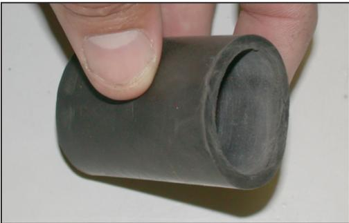
32. Cut a 2-1/2" length of hose from the provided silicone hose as shown.
