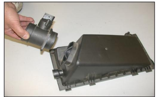
9. Remove the mass air sensor from the air cleaner cover as shown.
