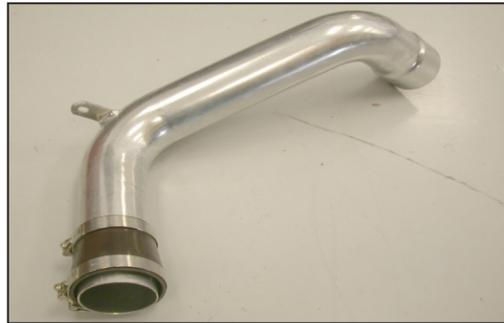
36. Install the silicone hose and hose clamps onto the K&N® cold air tube as shown.
