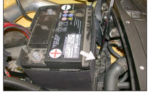
41. Reinstall the battery and the battery hold down block and secure as shown.
