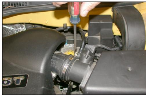
5. Loosen the hose clamp at the mass air sensor as shown.
