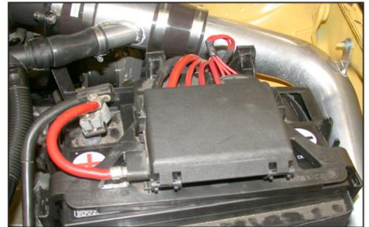
43. Reverse the removal process and slide the battery fuse/harness onto the battery cover as shown.
