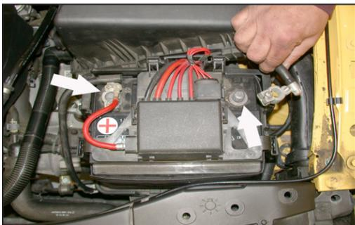
3. First disconnect the negative battery cable, then disconnect the positive battery cable as shown.
