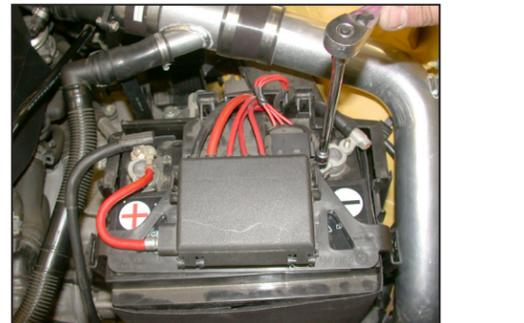
45. Reconnect the positive battery cable, and then the negative battery cable as shown.
