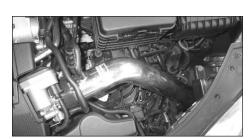
24. Align the new intake tube for best fit and clearance, then, firmly tighten the hose clamp and M6 and M10 nut.
