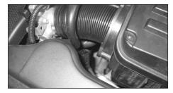
5. Unclip the temperature sensor electrical connector as shown.
