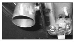
20. Mount the "L" bracket onto the thread of the front beam using the M10 washer and M10 nut supplied. Do not fully tighten at this moment.
