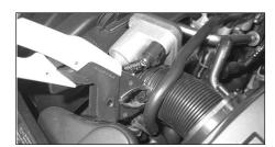
4. Remove the intake hose from the throttle body using a pair of pliers as shown.
