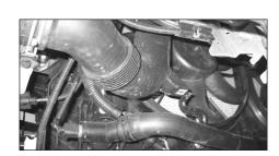
13. Unscrew the intake snorkel hose from the supprot bracket as shown.
