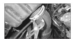
10. Unclip the intake snorkel hose from the resonator box using the pliers as shown.
