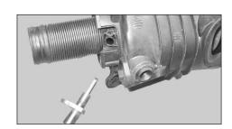
15. Remove the temperature sensor from the air box as shown.
