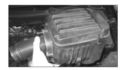
6. Remove the complete air box from the vehicle by pulling the air box upwards.
