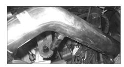
25. Reconnect the temperature sensor electrical connector and fit the wireloom of the temperature sensor onto the large wireloom.
