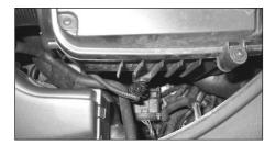
3. Unclip the wire loom from the side of the air box as shown.
