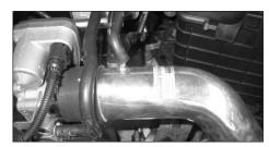
26. Fit the breather hose onto the new intake tube as shown.
