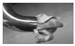
16. Clean the inside of the new intake tube with water and a towel.
