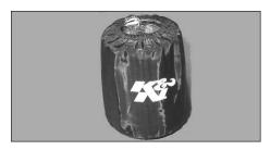
22. Fit the K&N Drycharger over the K&N Filter as shown. **NOTE:** The Drycharger's water repellant properties will last up to 2 years. See parts list to re-order Drycharger if necessary.
