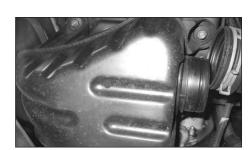
11. Remove the three bolts securing the resonator box to the vehicle.
