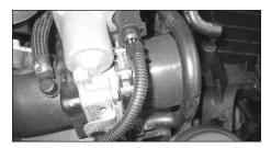
18. Fit the silicone sleeve onto the throttle body using the #40 hose clamp supplied.
