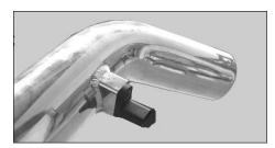
17. Mount the temperature sensor into the new intake tube using the M5 bolt supplied.
