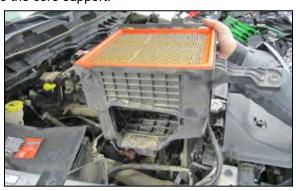
6. Lift up the lower air box to dislodge it from the mounting grommets and then remove it from the vehicle.
