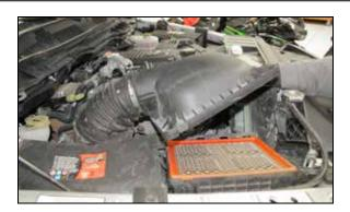
4. Release the two clips securing the air box lid and then remove the air box lid and intake tube from the vehicle.
