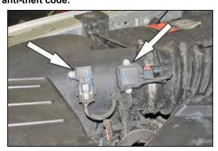
2. Disconnect the Mass air sensor and temperature sensor electrical connections, and then unhook the wiring harness from the air box.
