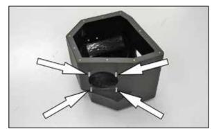
9. Install four of the provided 6mm studs into the K&N<sup>®</sup> air box as shown.
