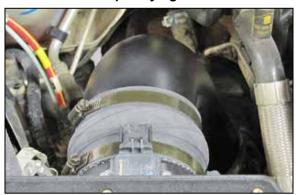
17. Install the K&N® intake tube into the factory turbo inlet hose and then connect the K&N® hose to the K&N® mass air sensor housing. Secure the intake tube with the hose clamps provided.
