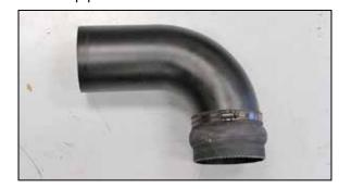
16. Install the provided silicone hose (08695) and hose clamps onto the K&N® intake tube as shown. NOTE: Do not completely tighten at this time.
