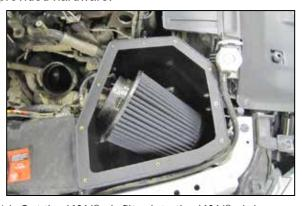
14. Set the K&N® air filter into the K&N® air box as shown.
