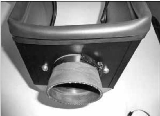
9. Install the air filter adapter onto the heat shield and secure with the provided hardware. Install the provided coupler (08186) onto the filter adapter and secure with the provided hose clamp.
