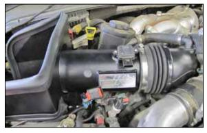
15. Install the K&N<sup>®</sup> intake tube into the factory inlet hose and align with the mounting bracket. Secure the tube with the factory hose clamp and hardware provided.
