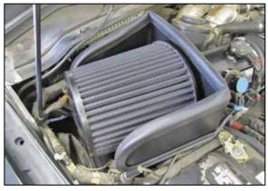
18. Install the K&N<sup>®</sup> air filter and secure with the provided hose clamp.
