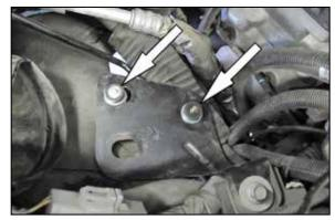
10. Install the two provided rubber mounted studs onto the air box mounting tray as shown. **NOTE: The fender washers should be placed on either side of the mounting tray with the rubber washers between each fender washer.**
