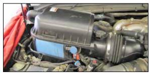
5. Release the two upper air box retaining clips and then remove the upper air box housing assembly as shown.
