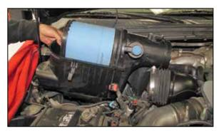
6. Lift up the lower air box to unhook it from the mounting grommets and then remove from the vehicle.
