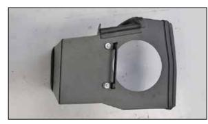
8. Install the tube mounting bracket (083167) onto the heat shield using the provided hardware.
