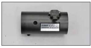
14. Install the mass air sensor into the K&N<sup>®</sup> intake tube and secure with the provided screws.
