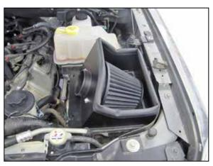
17. Set the heat shield assembly onto the lower air box and secure with the two remaining air box clins
