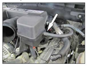
8. Disconnect the EVAP vent line from the intake plenum.
