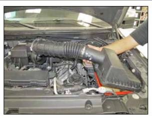
5. Remove the upper air box/intake hose assembly from the vehicle.
