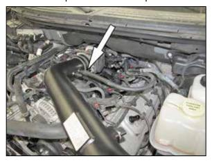
23. Install the provided hose mender into the provided EVAP hose and then install the hose mender into the factory EVAP hose. Connect the open end onto the fitting installed into the K&N® intake tube.
