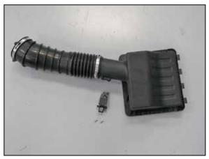
19. Remove the two screws securing the mass air sensor into the air box and then remove the sensor.
