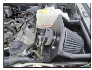
18. Install the provided hump coupler (08699) onto the filter adapter and secure with the provided hose clamp.
