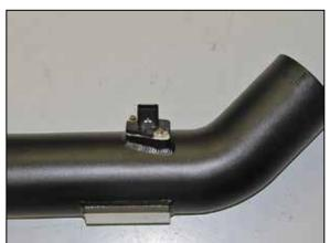
20. Install the mass air sensor into the K&N $^{\! \otimes}$  intake tube and secure with the provided hardware.
