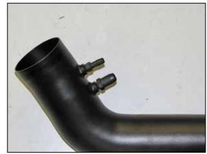
21. Install the two provided NPT vent fittings into the  $K\&N^{\tiny \circledcirc}$  intake tube as shown.
