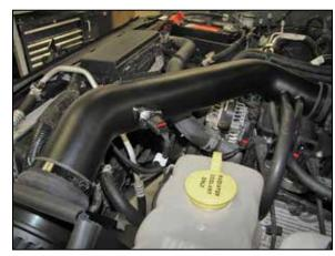
25. Connect the provided mass air sensor extension harness into the factory harness and then connect the open end to the mass air sensor.
