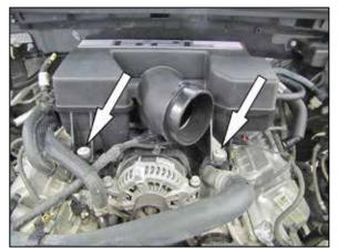
6. Remove the two bolts that secure the intake plenum.
