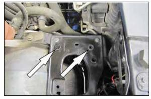
12. Remove the two air box mounting grommets shown.
