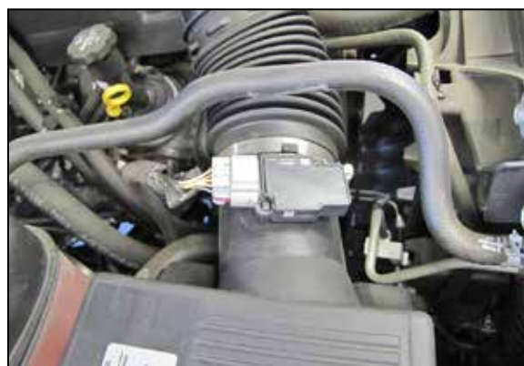
2. Disconnect the mass air electrical connection.
