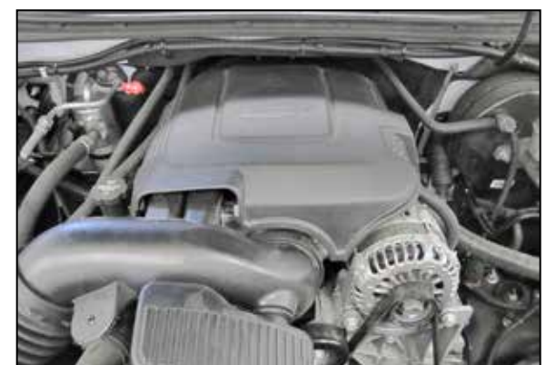
3. Lift up on the engine cover and remove as shown.
