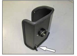
12. Install the provided heat shield mounting bracket (070015) onto the heat shield as shown using the provided hardware. NOTE: be sure to place one of the provided
