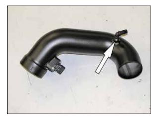
20. Install the provided 90° vent fitting into the K&N $^{\odot}$  intake tube as shown.
