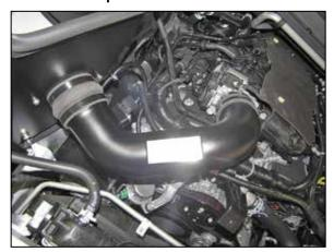
21. Install the K&N<sup>®</sup> intake tube into the hump coupler and then into the step coupler at the throttle body, adjust the tube for best fit and then secure with the provided hose clamps.
