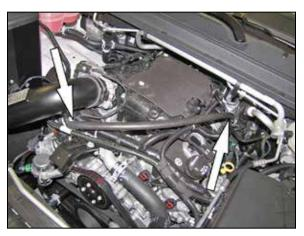
23. Install the crank case vent hose onto the fitting installed into the K&N<sup>®</sup> intake tube and then connect the hose mender into the fitting on the valve cover.
