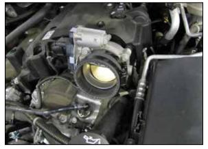
16. Install the provided coupler (08186) onto the throttle body and secure with the provided hose clamp.
