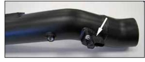
13. Remove the mass air sensor from the factory air filter housing and install the sensor into the K&N<sup>®</sup> intake tube using the provided hardware.
