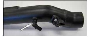
14. Install the 90° vent fitting into the K&N $^{\otimes}$  intake tube as shown.
