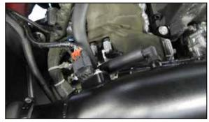
20. Using the provided vent hose, connect the factory vent to the 90° fitting installed into the K&N<sup>®</sup> intake tube. Reconnect the mass air sensor electrical connection.
