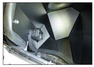
14. Install the heat shield assembly into the vehicle so the mounting grommet slides into the factory mounting hole. Slide the fresh air intake scoop into the opening in the heat shield and resecure to the core support with the factory clip. Secure the heat shield with the factory nut removed in step #9.
