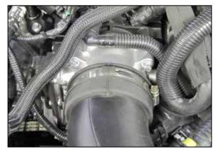
9. Loosen the hose clamp that secures the factory intake tube to the throttle body.
