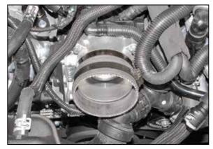
18. Install the provided silicone hose (08698) onto the throttle body and secure with the provided hose clamp.
