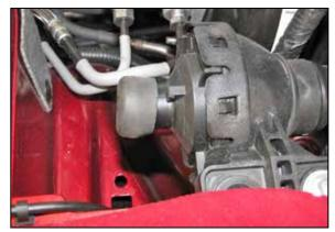
6. Install the provided cap onto the drum as shown.
