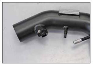
21. Install the mass air sensor into the K&N $^{\otimes}$  intake tube and secure with the provided hardware.
