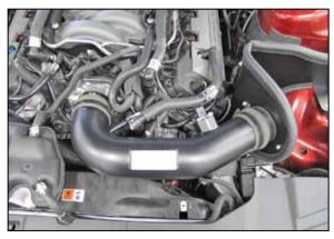
22. Install the K&N<sup>®</sup> intake tube into the silicone hoses, align for best fit and then secure with the provided hose clamps.
