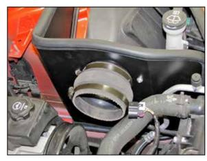
17. Install the silicone hose (08418) onto the filter adapter and secure with the provided hose clamp.
