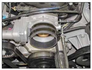
16. Install the silicone hose (08761) onto the throttle body and secure with the provided hose clamp.
