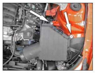
8. Remove the two air box retaining nuts shown.
