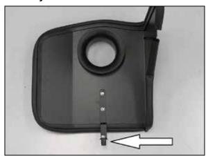
14. Install the inserted nut onto the heat shield mounting bracket using the provided hardware. Do not completely tighten at this time.
