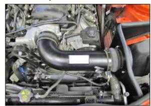
21. Install the K&N® intake tube assembly into the silicone hose at the filter adapter and then into the silicone hose at the throttle body and secure with the provided hose clamps.
