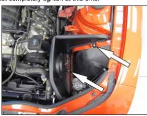
15. Install the heat shield assembly into the vehicle so the inserted nut goes into the air box mounting grommet hole and the tab goes onto the air box mounting stud. Secure the heat shield with the provided hardware.
