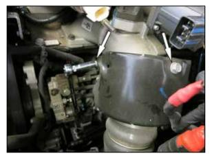
3. Remove the two bolts that secure the charge tube connection cover and then remove the cover.
