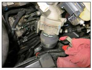
11. Install the provided hump coupler onto the charge tube with the clamps and then install on to the throttle body and secure with the hose clamps.
