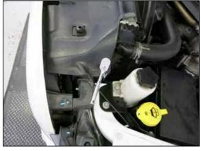
12. Using a ratchet with a long extension and a 11mm socket, tighten the clamps to secure the charge tube into the coupler at the intercooler.
