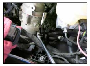
4. Loosen the hose clamp that secures the factory charge tube to the throttle body. Separate the charge tube from the throttle body.
