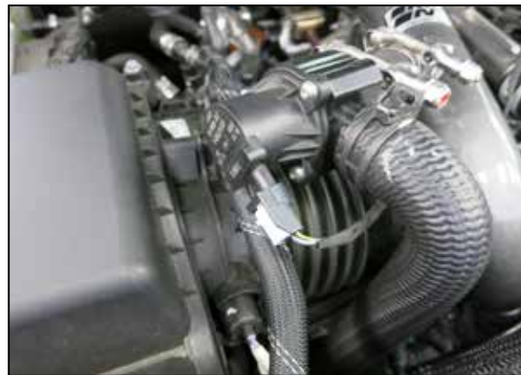
30. Reconnect the BOV valve electrical connection.
