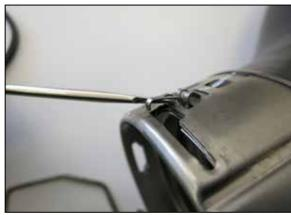
8. Using a small screwdriver or similar tool, bend the small tabs that retaining the locking clip onto the factory quick connect fitting and then remove the clip.
