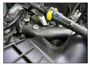
17. Connect the factory vent line to the quick connect fitting installed into the K&N charge tube and secure with the factory white locking clip.
