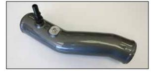
11. Using pipe sealant on the thread, install the quick connect vent fitting and 1/8npt pipe plug into the K&N charge tube.
