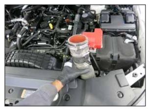
6. Remove the factory charge pipe from the vehicle.
