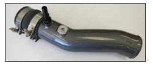
12. Install the provided hump coupler and clamps onto the K&N charge tube but do not tighten the clamps at this time.
