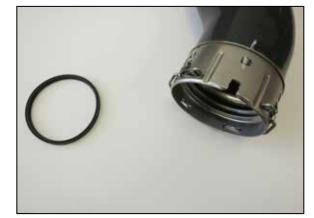
2. Loosen the hose clamp that secures the factory charge pipe coupler to the throttle body.
