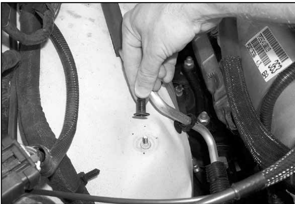
8. Unscrew plastic airbox retaining stud from vehicle as shown.
