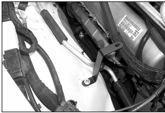
10. Mount the provided "Z" bracket onto the inner fender well as shown. Do not tighten completely.
