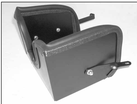
12. Install the provided twist bracket onto heat shield as shown. Do not tighten completely.
