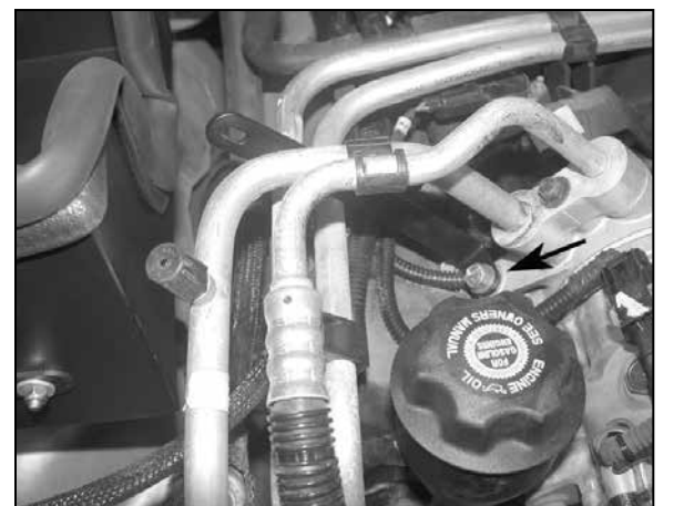
19. Install the tube-mounting bracket onto the A/C compressor with the bolt removed in step #18.
