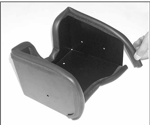
9. Apply the provided trim seal to the heat shield as shown.
