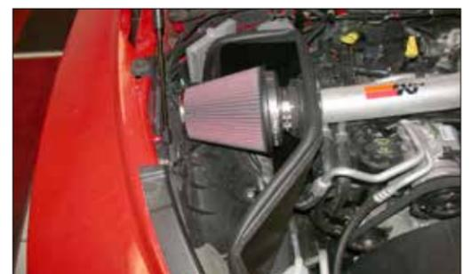
26. Install the air filter assembly onto the K&N® intake tube and secure with the provided hose clamp as shown.
