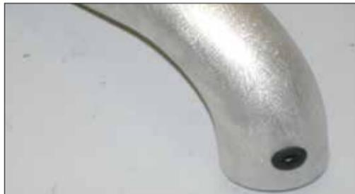
18. Install the provided grommet into the K&N® intake tube as shown.
