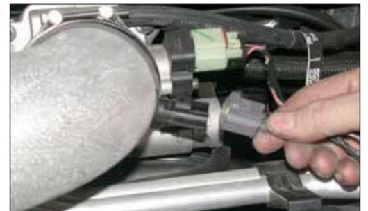
22. Reconnect the air temperature sensor electrical connection as shown.
