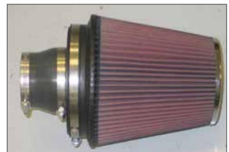
25. Install the silicone hose (084055) onto the air filter adapter as shown and secure with the provided hose clamp as shown.
