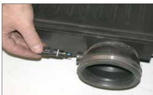
17. Twist the air temperature sensor counter clockwise and remove it from the stock intake plenum.
