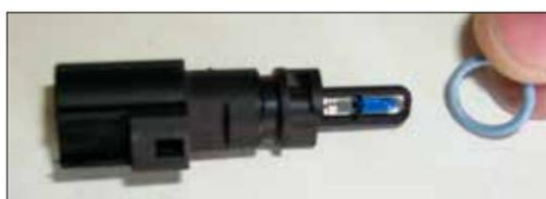
19. Remove the O-ring from the air temp. sensor as shown.
