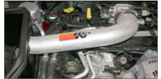
21. Install the K&N® intake tube into the throttle body hose and position so the mounting bracket aligns with the tube mounting stand off and then secure with the provided hardware.
