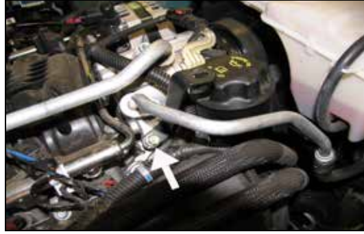
16. Install the "Z" bracket (020019) onto the A/C compressor and secure with the bolt removed in step #15.
