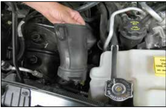
10. Remove the fresh air duct from the radiator core support as shown.
