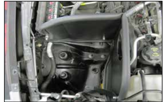
22. Install the heat shield assembly into the vehicle so that the two small "L" brackets align with the threaded stud on the inner fender and the ECU mounting stud.
