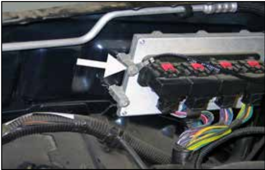
11a. On 2008 and later vehicles, remove the front-upper ECU mounting bolt shown. NOTE: This bolt will be reused in a later step.
