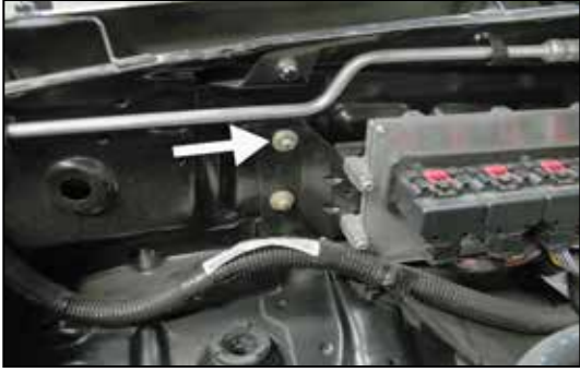
11. On 2007 model year vehicles, remove the front-upper ECU mounting nut shown. NOTE: This nut will be reused in a later step.
