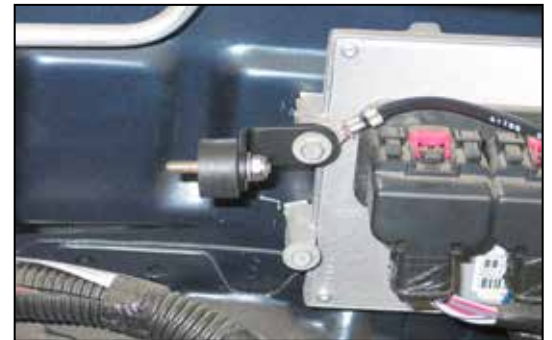
21b. On 2008 and later vehicles, attach the "L" bracket assembly from step #21a. to the ECU using the factory bolt removed in step #11a. NOTE: Be sure to place the ground wire between the bracket and ECU as shown.
