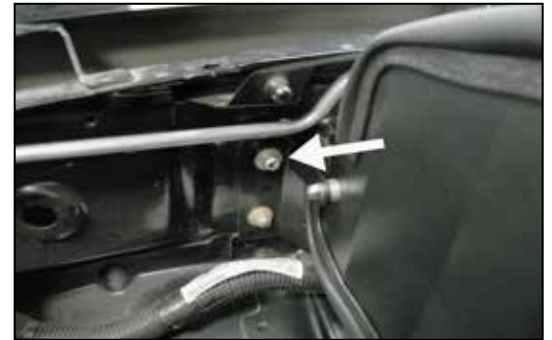
23. On 2007 model year vehicles, secure the upper heat shield mounting bracket with the nut removed in step #11.
