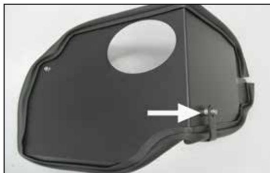
20. Install the small "L" bracket (070742) onto the heat shield as shown using the spacer and hardware provided. NOTE: Place the spacer between the heat shield and bracket.
