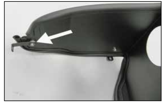
21. On 2007 and later vehicles, install the remaining small "L" bracket (06464) onto the heat shield with the provided spacer and hardware. NOTE: Place the spacer between the heat shield and bracket.
