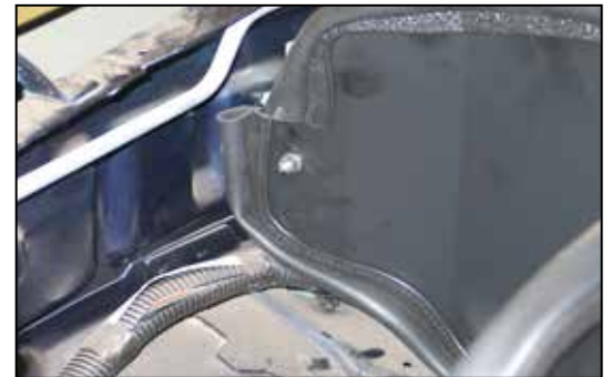
23a. On 2008 and later vehicles, secure the heat shield to the rubber mounted stud installed during step #21b.
