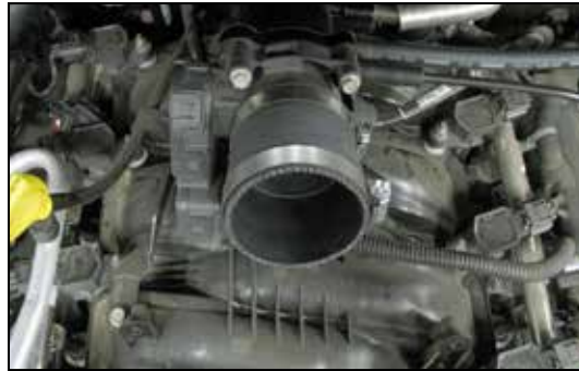
17. Install the silicone hose (08096) onto the throttle body and secure with the provided hose clamp.
