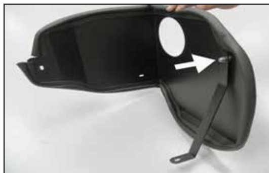
19. Install the large "L" bracket (020020) onto the heat shield and secure with the provided spacer and hardware. NOTE: Place the spacer between the heat shield and bracket.
