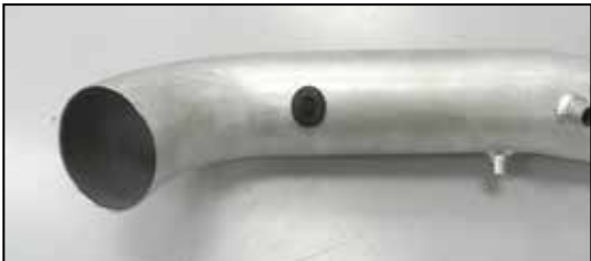
12. Install the provided grommet into the K&N® intake tube as shown.
