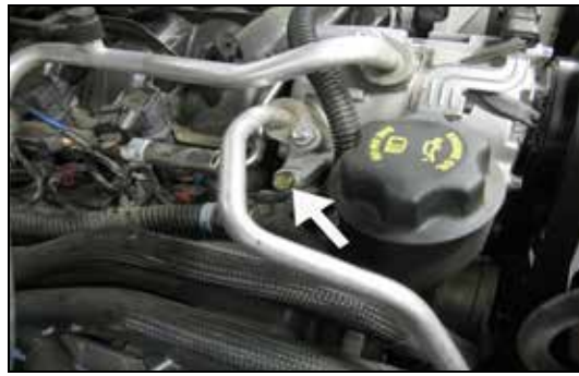
15. Remove the A/C mounting bolt shown. NOTE: This bolt will be reused.
