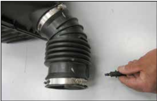
13. Remove the air temperature sensor from the stock intake tube. NOTE: Take care removing the air temperature sensor as it is very fragile.
