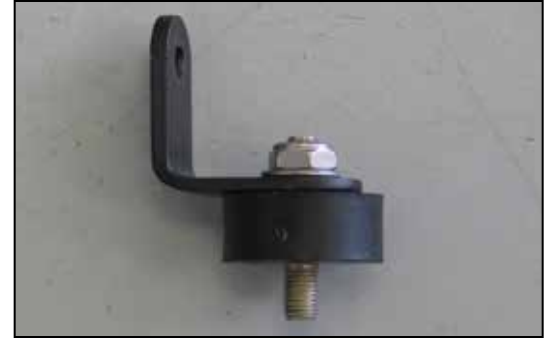
21a. On 2008 and later vehicles, attach the rubber mounted stud to the small "L" bracket (070066) with the provided hardware as shown.
