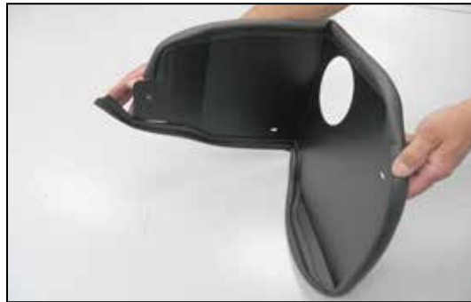
18. Install the provided edge trim onto the heat shield. NOTE: Some trimming of the edge trim may be necessary.
