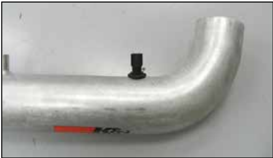
14. Install the air temperature sensor into the grommet installed in the K&N® intake tube during step #12.
