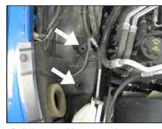
6. Pull the two airbox mounting grommets shown from the inner fender.
