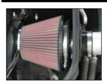
26. Install the air filter assembly onto the K&N® intake tube and secure with the provided hose clamp.
