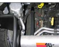
23. Install the provided silicone hose onto the fitting on the K&N® intake tube and then attach the open end onto the hose to the factory crankcase tube.
