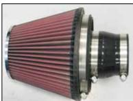
25. Install the silicone hose (08724) onto the air filter adapter as shown and secure with the provided hose clamp.
