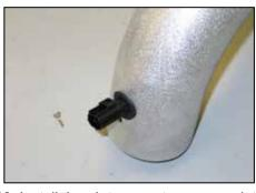
20. Install the air temperature sensor into the grommet installed into the K&N® intake tube in step #17
