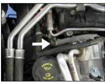
14. Remove the rear, lower A/C compressor mounting bolt shown.
