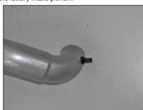
20. Install the inlet air temperature sensor into the grommet installed into the K&N® intake tube. NOTE: Remove the factory sealing O-ring from the sensor before installation.
