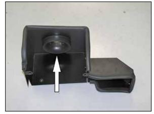
12. Install the K&N<sup>®</sup> air filter adapter into the heat shield and secure with the provided hardware.
