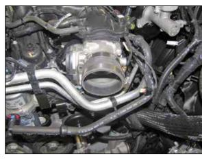
17. Install the provided silicone hose (08690) onto the throttle body and secure with the provided hose clamp.
