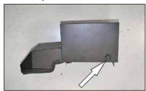
11. Install the factory rubber mounting grommet into the K&N® heat shield as shown.
