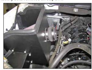
16. Install the provided silicone hose (08699) onto the filter adapter and secure with the provided hose clamp.
