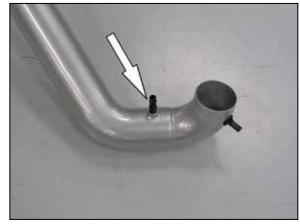
21. Install the provided vent fitting into the  $K\&N^{\otimes}$  intake tube as shown.
