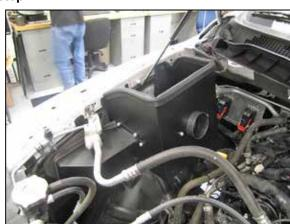
15. Set the heat shield into position on the factory air box mounting bracket and then secure with the factory bolts removed on step #14.
