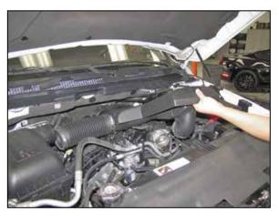
5. Lift up the intake plenum to dislodge it from the mounting grommets and then remove the plenum from the vehicle.
