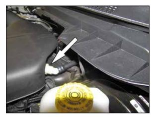
3. Disconnect the crank case vent from the intake plenum.
