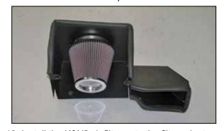
13. Install the K&N® air filter onto the filter adapter and secure with the provided hose clamp.
