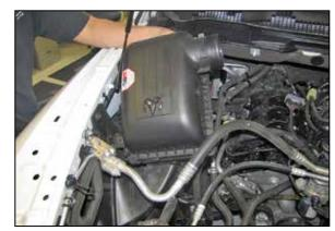
6. Lift the air box assembly off of the mounting studs and then remove the air box from the vehicle. NOTE: K&N Engineering, Inc., recommends that customers do not discard factory air intake.
