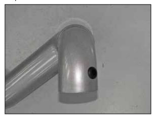
18. Install the provided grommet into the  $K\&N^{\otimes}$  intake tube.
