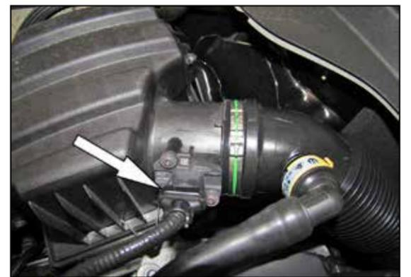
5. On vehicles equipped with a humidity sensor, Disconnect the wiring harness from the sensor.
