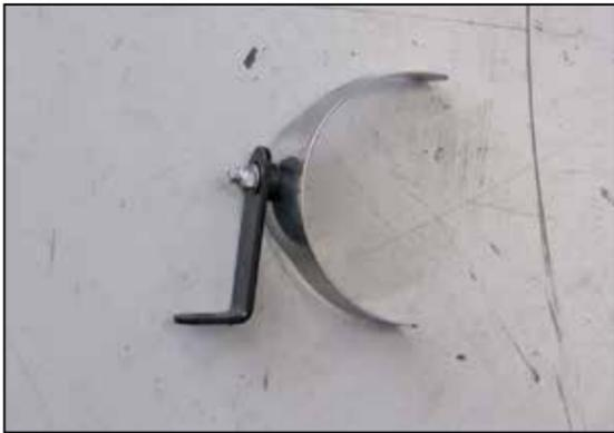
22. Assemble the saddle onto the provided bracket (070109) as shown using the provided hardware.
