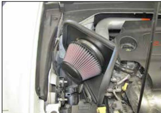
28. Install the filter assembly onto the K&N® intake tube and adjust for best fit and then secure with the provided hose clamp.
