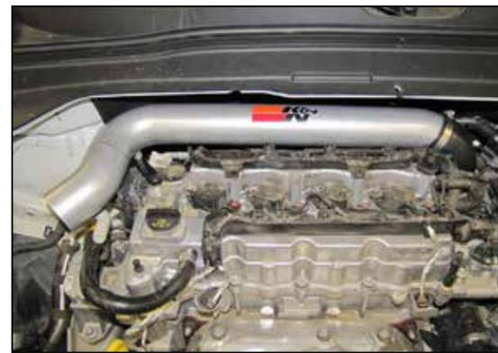
17. Install the K&N intake tube assembly into the coupling hose and align the bracket with the mounting lug on the valve cover. Tighten the hose clamps but do not secure the bracket to the valve cover.
