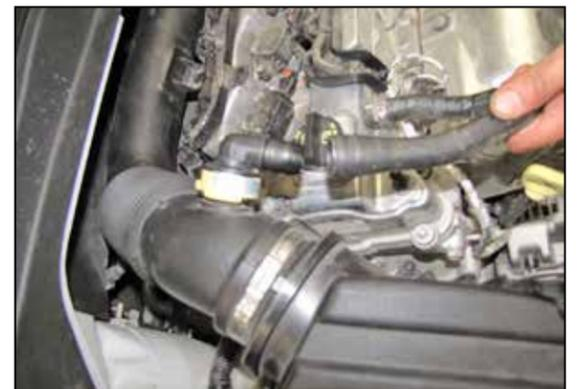
6. Disconnect the crank case vent hose from the fitting in the intake tube.
