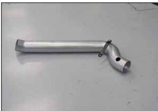
11. Install the tube mounting bracket (064335) onto the K&N intake tube as shown using the provided hardware.
