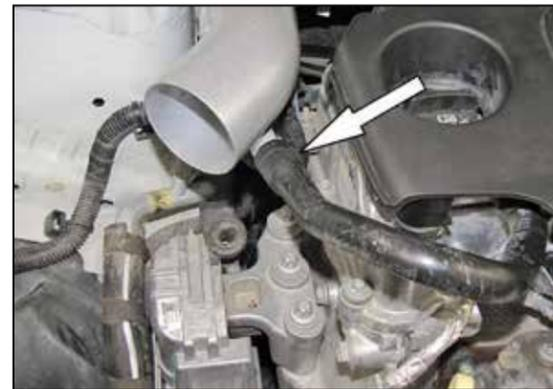
20. Connect the crank case vent hose to the fitting installed into the K&N intake tube.
