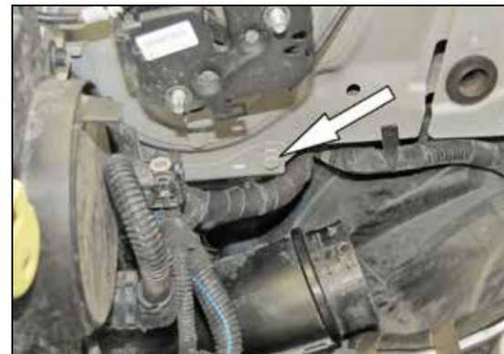
21. Remove the inner fender bolt shown.
