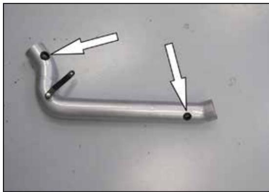
12. Install the two provided grommets into the K&N intake tube as shown.
