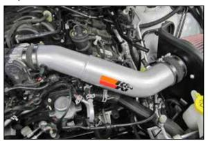
19. Install the K&N® intake tube into the coupler at the throttle body and then into the hump coupler, adjust the tube for best fit and then secure with the provided hose clamps.
