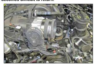
18. Install the provided step coupler onto the throttle body and secure with the provided hose clamp.
