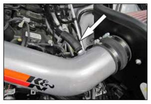
21. Install the provided crank case vent hose onto the fitting installed into the K&N® intake tube and then connect the other end to the factory crank case vent tube.
