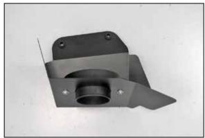
10. Install the filter adapter into the K&N® heat shield and secure with the provided hardware as shown.
