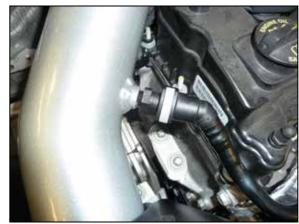
21. Reconnect the PCV to the Quick connect fitting installed into the  $K\&N^{\tiny \circledcirc}$  intake tube.
