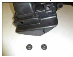
6. Remove the two mounting grommets from the factory air filter housing.
