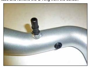
11. Install the provided grommet and quick disconnect fitting into the K&N<sup>®</sup> intake tube as shown.
