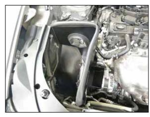
17. Install the heat shield into the vehicle as shown so the mounting studs insert into the grommets.
