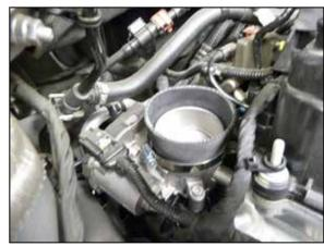
18. Install the provided coupler onto the throttle body and secure with the provided hose clamp.
