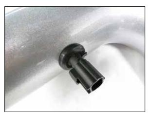
12. Install the IAT sensor into the grommet installed into the  $K\&N^{\otimes}$  intake tube.
