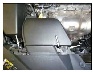
3. Remove the three bolts shown that secure the fresh air intake duct and then remove the duct from the engine.
