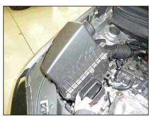
5. Pull the air filter housing straight up and remove it from the vehicle.
