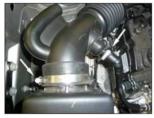
4. Push in the lock for the PCV vent and then disconnect the PCV vent from the intake tube. Loosen the hose clamp that secures the intake tube to the air filter housing and then disconnect the hose from the housing.
