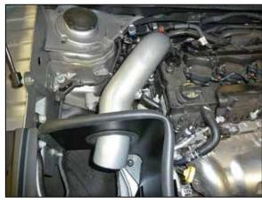
19. Install the K&N® intake tube into the heat shield and then into the coupler, adjust the tube for best fit and then secure with the provided hose clamp.
