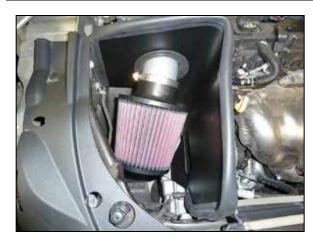
22. Install the K&N® air filter onto the intake tube and secure with the provided hose clamp. NOTE: Drycharger® air filter wrap; part # RX-4990DK is available to purchase separately. To learn more about Drycharger® filter wraps or look up color availability please visit http://www.knfilters.com<sup>®</sup>.
