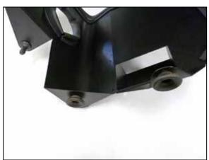
16. Install the two factory air filter housing mounting brackets onto the heat shield as shown.
