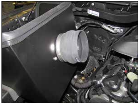
9. Install the provided coupler (08418) onto the filter adapter and secure with the provided hose clamp.
