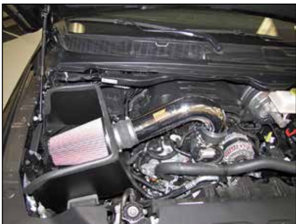
15. Reconnect the vehicle's negative battery cable. Double check to make sure everything is tight and properly positioned before starting the vehicle.
