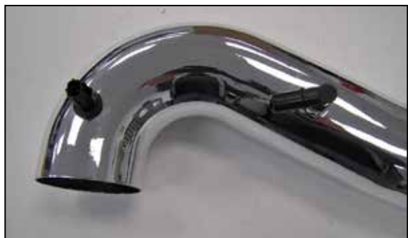
11. Install the inlet air temperature sensor into the K&N® intake tube using the provided grommet. Install the 90° NPT fitting onto the K&N® intake tube as shown. NOTE: Plastic NPT fittings are easy to cross thread. Install the vent fitting “hand” tight, then turn it two complete turns with a wrench.
