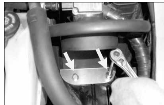
20. Tighten the hex bolts on the heat shield as shown.
