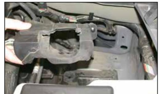
8. Pull firmly on the air inlet duct to dislodge it from core support and remove from the vehicle.
