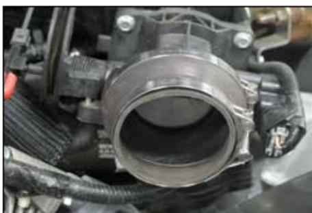
10. Install the silicone hose (084034) onto the throttle body and secure with the provided hose clamp as shown.
