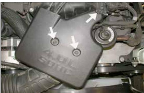
3. Remove the three engine cover mounting bolts shown.
