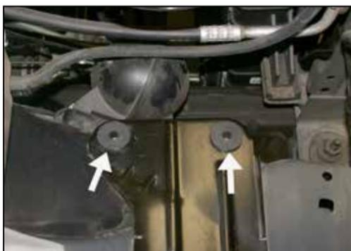
18. Install the two provided threaded inserts into the lower air box mounting plate at shown.
