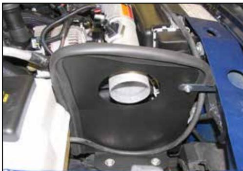
19. Install the heat shield assembly into the vehicle so the bracket lines up with the factory hole in the core support and the holes in the heat shield line up to the inserts installed in step #18. Secure the heat shield with the provided hardware.
