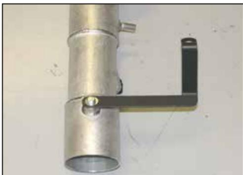
13. Install the provided tube mounting bracket (010081) onto the K&N® intake tube with the provided hardware as shown.
