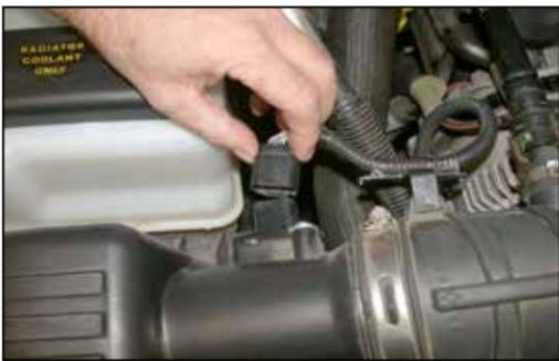
2. Disconnect the mass air sensor electrical connection and separate the harness from the stock intake tube wiring harness clip.
