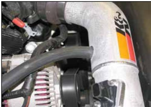
20. Install the provided crank case vent hose onto the fitting at the valve cover then attach the other end to the port on the K&N® intake tube.
