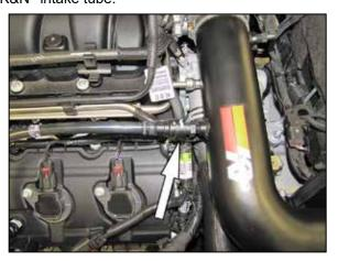
23. Connect the factory crank case vent to the quick connect fitting installed into the K&N<sup>®</sup> intake tube as shown.
