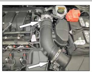
5. Loosen the two hose clamps which secure the factory intake tube to the throttle body and factory air box. Remove the factory intake tube from the vehicle.
