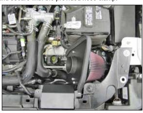
14. Install the heat shield assembly into the vehicle so that the mounting studs go into the air box mounting grommets.
