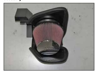
13. Install the K&N<sup>®</sup> air filter onto the filter adapter and secure with the provided hose clamp.
