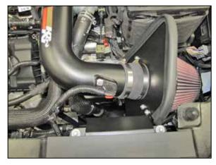
24. Connect the mass air sensor electrical connection.
