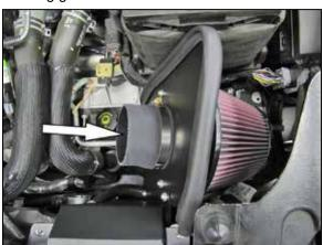
15. Install the provided silicone hose (08496) onto the filter adapter and secure with the provided hose clamp
