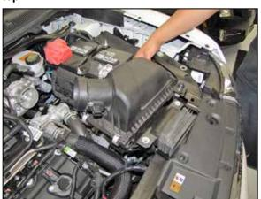
8. Lift up the air box to dislodge it from the mounting grommets and then remove it from the vehicle.
