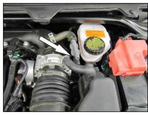
4. Disconnect the EVAP vent line from the check valve as shown.
