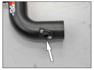
19. Install the mass air sensor into the K&N $^{\!0}$  intake tube and secure with the provided hardware.
