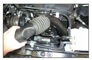
5. Release the two tabs that secure the fresh air duct to the inlet in the core support and remove the fresh air duct.
