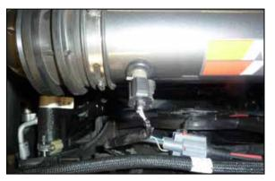
17. Reconnect the inlet temperature sensor electrical connection.
