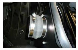
13. Install the hump coupler onto the filter adapter and secure with the provided hose clamp.
