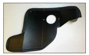
6. Install the provided edge trim onto the heat shield as shown, some trimming of the edge trim will be necessary.
