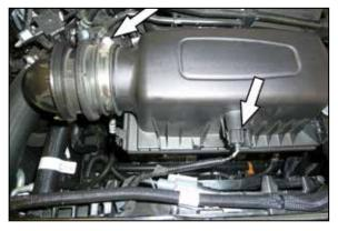
2. Loosen the hose clamp that secures the intake hose to the air filter housing and disconnect the hose from the housing. Disconnect the inlet air temperature sensor electrical connection 3.Release the spring clips that secure the upper air filter housing to the lower housing and then remove the upper housing and factory air filter.
