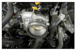
13. Install the provided straight coupler onto the throttle body and secure with the provided hose
