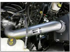
17. Install the Intake tube into the coupler at the throttle body and then into the coupler at the filter adapter, adjust the tube for best fit and secure with the provided hose clamps.
