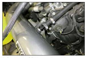
18. Connect the CCV hose to the quick connect fitting installed onto the intake tube.
