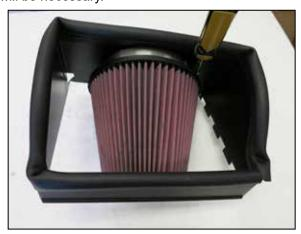
11. Install the air filter ono the filter adapter and secure with the provided hose clamp.
