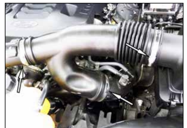
3. Loosen the three hose clamps that secure the factory intake tube and then remove the intake tube from the vehicle.
