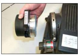
7. Loosen the hose clamp on the air cleaner then remove the mass air sensor as shown.
