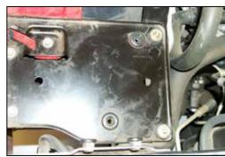
9. Install the rubber mounted studs as shown and tighten firmly by hand.
