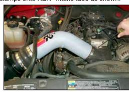
16. Install the K&N® intake tube into the angled hose, then, slide the other end into the hump hose. Adjust everything for best fit and clearance and tighten all hose clamps as shown.
