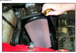
18. Install the K&N® air filter onto the mass air adapter and secure it with the provided hose clamp as shown.
