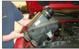
6. Pull firmly upwards to remove the air cleaner assembly as shown.
