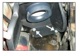
13. Secure the heat shield to the rubber mounted studs using the provided hardware but do not tighten at this time
