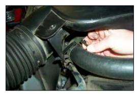
4. Unclip the radiator hose from the stock intake tube as shown.
