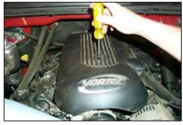
20. Reinstall the engine cover and secure it with the stock hex bolt.
