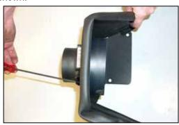
11. Using the provided hardware assemble the mass air adapter, heat shield, gaskets and the stock mass air sensor as shown.
