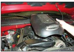
2. Remove the bolt that secures the engine cover, then, remove the engine cover as shown.
