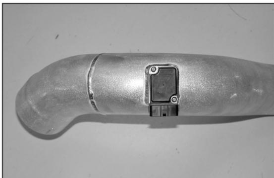
14. Install the mass air sensor into the K&N® intake tube and secure with the provided hardware as shown.
