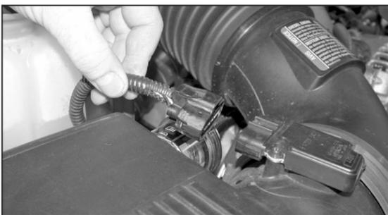
2. Depress the locking tab on the mass air sensor electrical connector, and then disconnect the electrical connection.
