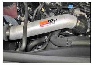
17. Install the K&N<sup>®</sup> intake tube into the coupling hoses and then adjust the tube for best fit. Secure the hoses and tube with the provided hose clamps.
