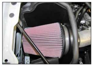
19. Install the K&N<sup>®</sup> air filter and secure with the provided hose clamp.
