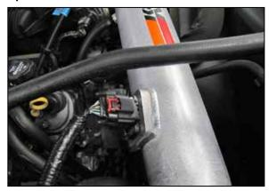
20. Reconnect the mass air sensor sensor electrical connections.
