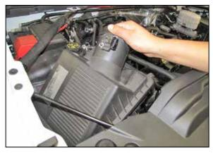
6. Lift up the air box to dislodge it from the mounting grommets, and then remove it from the vehicle as shown.
