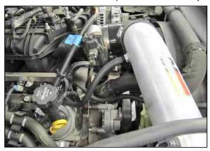
18. Install the provided crank case vent hose onto the fitting installed into the  $K\&N^{\textcircled{o}}$  intake tube and then onto the valve cover port. Secure the hose to the valve cover port with the provided hose clamp.
