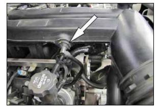
4. Disconnect he crank case vent hose from the intake tube plenum.
