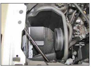
11. Install the heat shield assembly onto the air filter housing mounting plate location and secure with three of the factory bolts from step #8.
