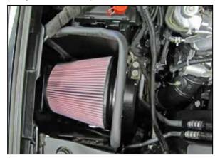
9. Flex the heat shield inward towards the engine then install the K&N® air filter onto the filter adapter and secure with the provided hose clamp. Secure the heat shield with two of the remaining factory bolts from step #5.
