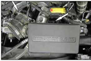
3. Remove the nut that secures the intake plenum to the Engine and then loosen the hose clamp that secures the plenum to the turbo inlet. Remove the intake plenum from the vehicle.
