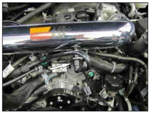
19. Rotate the crank case vent line and fitting so it aligns with the quick connect fitting and then connect.
