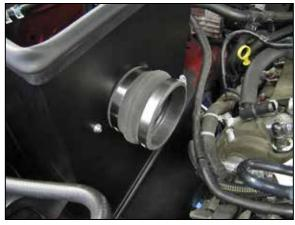
17. Install the provided hump coupler (08699) onto the heat shield and secure with the provided hose clamp.
