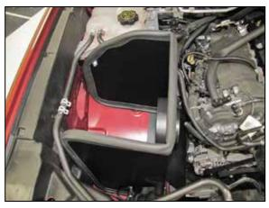
12. Install the heat shield assembly into the vehicle and secure with the factory coolant reservoir nut and air box mounting nut.
