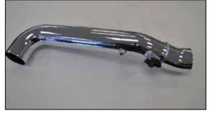
13. Remove the mass air sensor from the factory air filter housing and install the sensor into the  $K\&N^{\odot}$  intake tube using the provided hardware.
