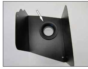
7. Install the filter adapter into the K&N $^{\odot}$  heat shield and secure with the provided hardware.
