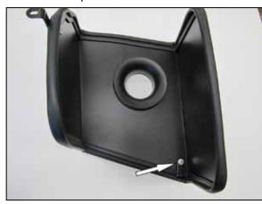
10. Install the provided heat shield mounting bracket (070015) onto the heat shield using the provided bardware and appear
