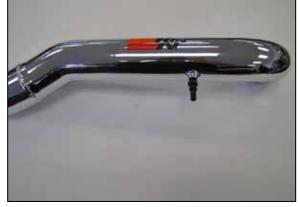
14. Install the quick connect fitting into the K&N $^{\mbox{\tiny \$}}$  intake tube as shown.
