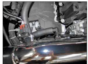
20. Using the provided vent hose, connect the factory vent to the  $90^{\circ}$  fitting installed into the
