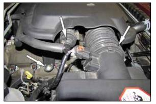
2. Loosen the hose clamp that secures the intake hose to the air filter housing. Using a screwdriver, unlock the small clamp that secures the vent line to the connector and then disconnect the vent line. Remove the bolt securing the intake plenum to the engine. 3. Remove the oil fill cap and loosen the hose clamp securing the intake hose to the throttle body. Remove the bolt securing the intake plenum to the engine.
