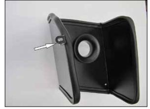
9. Install the provided heat shield mounting bracket (07805) onto the heat shield using the provided hardware and spacer.
