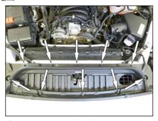
6. Release the ten retaining clips that secure the upper radiator valence and then remove the valence from the vehicle.
