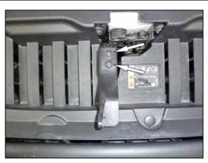
5. Remove the two bolts that secure the hood release arm to the hood latch and then remove the
