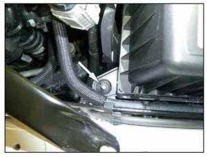
9. Remove the nut that secures the air filter housing. Unhook the wiring harness from the filter housing and then remove the air filter housing from the vehicle.
