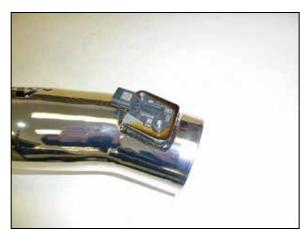
21. Remove the mass air sensor from the factory housing. Install the mass air sensor into the K&N® intake tube and secure with the provided hardware.
