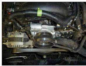
19. Install the provided reducer coupler onto the throttle body and secure with the provided hose clamp.
