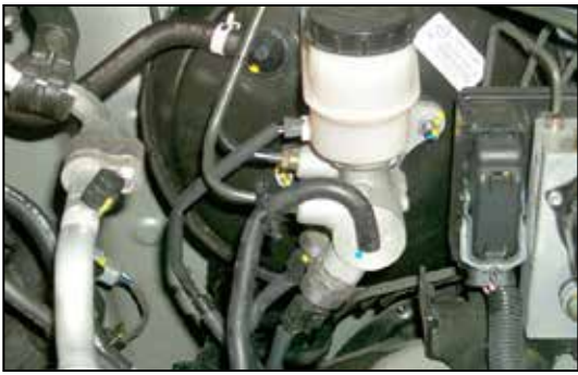
9a. On four wheel drive vehicles, secure the front differential vent tube to the front brake hardline as shown with the provided tie wrap.
