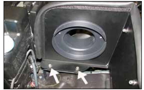
21. Install the heat shield into the vehicle and secure it to the rubber mounted studs using the provided hardware as shown, but do not tighten at this time.
