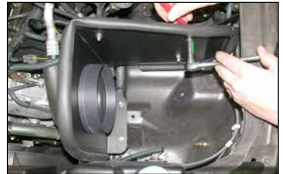
24. Adjust everything for best fit and clearance, then, tighten all hardware at this time.
