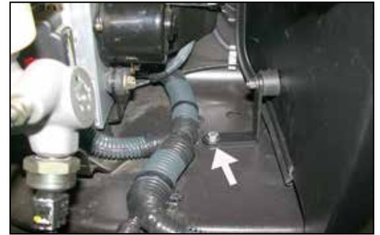
21. Install the heat shield into the vehicle and secure it to the rubber mounted studs using the provided hardware as shown, but do not tighten at this time.
