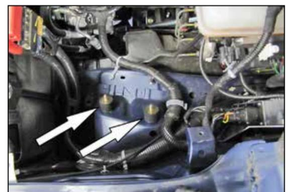
5. Install the two provided rubber mounted studs into the air filter housing mounting locations as shown.
