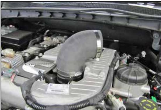
11. Install the provided coupler hose (08502) onto the turbo inlet and secure with the provided hose clamp.
