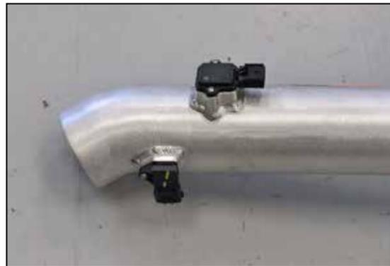
14. Install the sensors into the K&N® intake tube and secure with the provided hardware.
