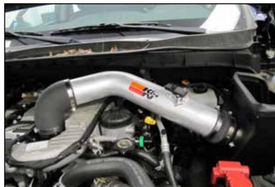
15. Install the K&N® intake tube into the coupler at the filter adapter and then into the hose at the turbo inlet, adjust the tube for best fit and then secure with the provided hose clamps.
