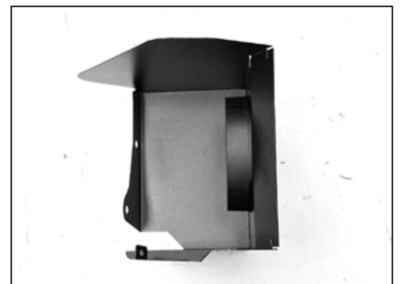
6. Install the provided filter adapter into the heat shield and secure with the provided hardware.
