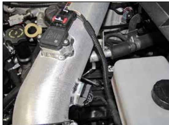
15. Reconnect the mass air sensor and inlet air temperature sensor electrical connections.
