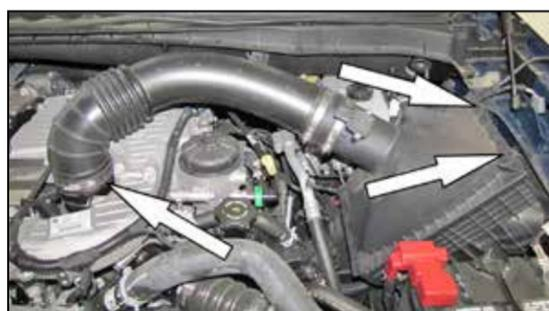
3. Loosen the hose clamp that secure the intake tube to the turbo inlet and then release the two clam shell clips that secure the upper air filter housing. Remove the upper air filter housing and intake tube from the vehicle.
