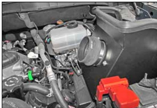
12. Install the provided coupler hose (08698) onto the filter adapter and secure with the provided hose clamp.
