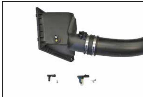
13. Remove the two sensors from the stock air filter housing.
