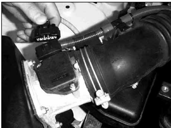
2. Disconnect the mass air sensor electrical connection.
