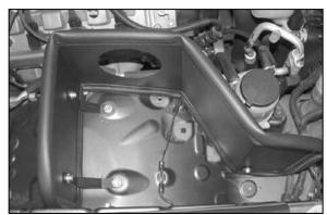
11. Install the heat shield onto the vehicle then secure to brackets with the provided hardware.
