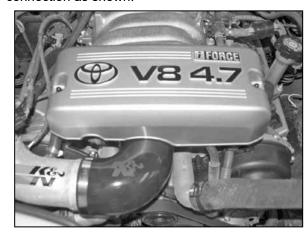
26. Reinstall the throttle body cover as shown. Note: On Lexus GX470 models the Passenger side engine compartment panel will fit, light pressure will need to be applied down so the clips can be engaged. The cover can be left off if desired.
