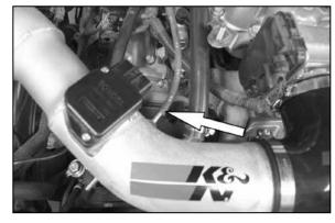
18. Connect the factory fuel pressure vent hose onto the K&N® intake tube as shown.
