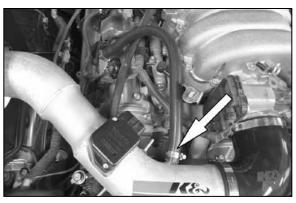
17. Remove the factory crank case vent hose from valve cover and then install the supplied vent hose onto the valve cover and K&N® intake tube and secure with the supplied hose clamp as shown.
