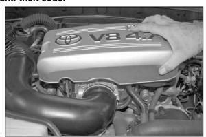
2. Loosen the two nuts that secure the throttle body cover, then remove the throttle body cover. Note: The cover may be different. On Lexus GX470 models, the passenger side engine compartment cover panel will also need to be removed.
