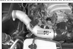
16. Install the K&N® intake tube into the silicone hose at the throttle body and align the mounting boss with the mounting bracket installed in step #12. Secure with the provided hardware.
