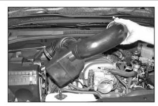
5. Loosen the hose clamp at the throttle body and air box, then remove intake tube from vehicle.
