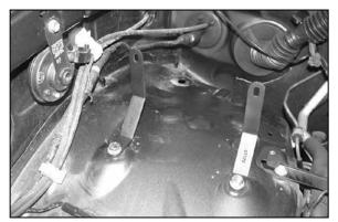
9. Mount the two provided brackets onto the vehicle with the provided hardware. NOTE: Bracket (07172) mounts closest to engine.
