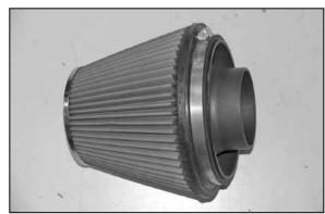
20. Install the filter adapter into the air filter as shown and secure with the provided hose clamp. NOTE: Drycharger® air filter wrap; part # RF-1048DK is available to purchase separately. To learn more about Drycharger® filter wraps or look up color availability please visit http://www.knfilters.com®.
