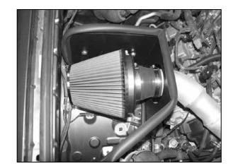
22. Install the air filter assembly onto the K&N® intake as shown and secure with the provided hose clamp.
