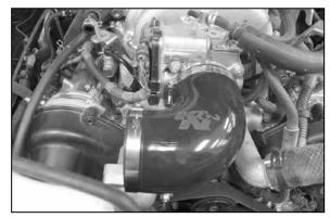
13. Install the provided silicone hose (084095) onto the throttle body with the provided hose clamp. NOTE: The synch bolt in the #350 hose clamp at the throttle body will need to be replaced with the longer synch bolt supplied.
