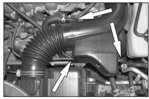
4. Remove the three vent lines from the air intake resonator as shown.
