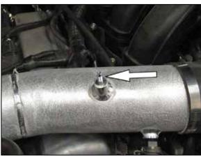
33. Install the engine cover mounting stud into the  $K\&N^{\circledast}$  intake tube.
