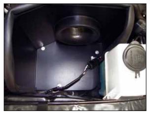
22. Route the secondary air wiring harness through the heat shield and reconnect the electrical connection.
