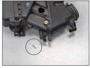
32. Remove the engine cover mounting stud from the air filter housing.
