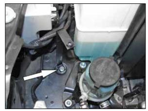
17. Install the provided secondary air pump mounting bracket (083169) onto the inner fender using the provided hardware. NOTE: The nut and washer will be accessed
