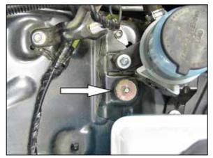
11. Install the provided 8mm rubber mounted stud into the intake resonator mounting location as shown.
