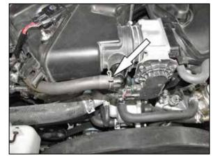
8. Release the spring clamp securing the crank case vent hose and then disconnect the crank case vent hose.
