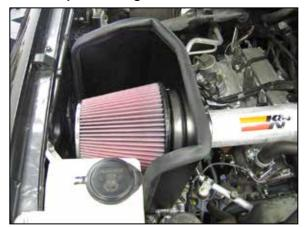
35. Install the K&N<sup>®</sup> air filter and secure with the provided hose clamp.
