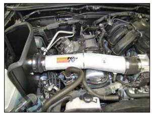
28. Install the K&N<sup>®</sup> intake tube into the silicone hose at the filter adapter far enough to gain clearance into the silicone hose at the throttle body, then install the tube into the throttle body silicone hose and secure it with the provided hose clamps. **NOTE: Do not completely tighten at this time.**
