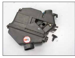
26. Remove the two screws securing the mass air sensor into the air filter housing and then remove the mass air sensor from the housing.
