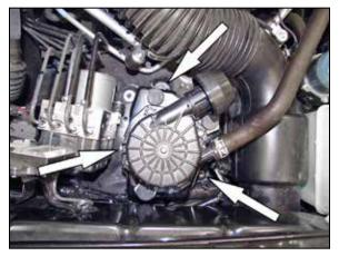
4. Remove the three bolts securing the secondary air pump and then disconnect the electrical connection and remove the secondary air pump from the engine compartment.
