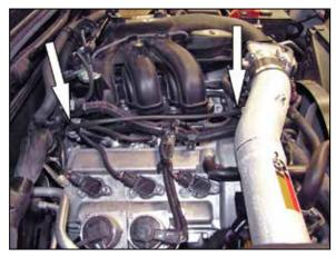
30. Connect the provided fuel pressure vent hose to the fuel pressure regulator and then connect the open end to the fitting installed into the K&N<sup>®</sup> intake tube.
