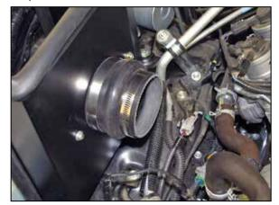
24. Install the provided silicone hose (084079) onto the filter adapter and secure with the provided hose clamp.
