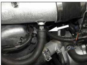
29. Connect the crank case vent hose to the fitting
