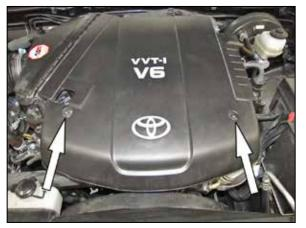
2. Remove the two nuts which secure the engine cover and then lift off the engine cover.
