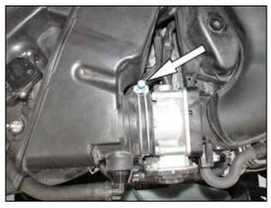
7. Loosen the hose clamp securing the intake hose to the throttle body.
