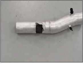
27. Install the mass air sensor into the K&N $^{\mbox{\tiny @}}$  intake tube and secure with the provided hardware.
