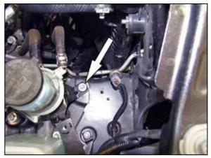
18. Remove the power steering reservoir mounting bolt shown.
