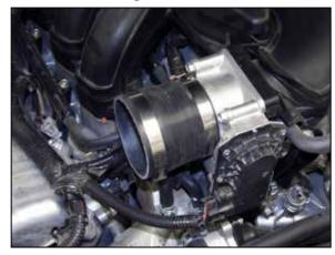
23. Install the provided silicone hose (08429) onto the throttle body and secure with the provided hose clamp.
