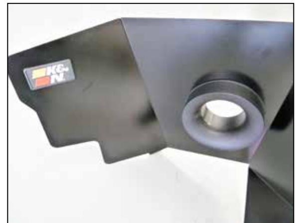
10. Install the filter adapters and K&N badges onto the heat shields using the provided hardware.
