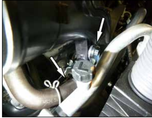
6. Disconnect the PCV hose from the driver side lower intake tube, Remove the intake tube mounting bolt then loosen the hose clamp securing the intake tube to the turbo inlet and remove the tube from the vehicle.
