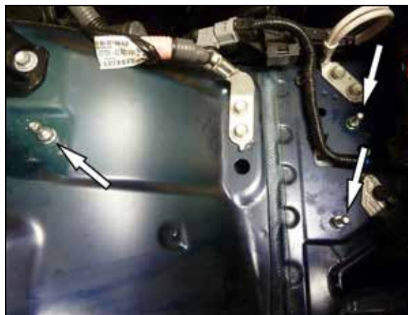
8. Remove the three air filter housing mounting studs from both the left and right sides.
