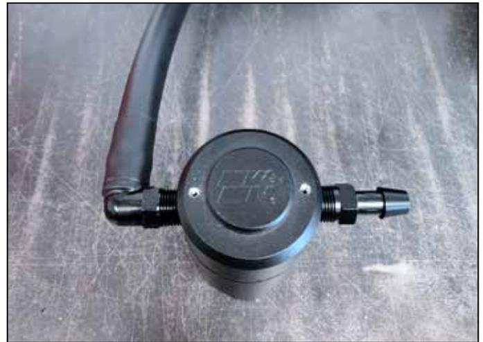
4. Assemble the hose fittings to the top of the air/oil separator. Assemble the long hose on the passenger side going to PCV valve. Assemble straight barb fitting to existing 90 degree elbow going to intake manifold. We recommend using PTFE tape on the fittings to ensure a proper seal.
