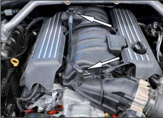
2. Remove the factory PCV hardline from both rubber connection points. You may need to twist the rubber ends with pliers to break seal on connections.
