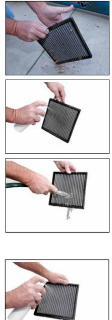
Use only K&N<sup>®</sup> cabin air filter Refresher<sup>™</sup> kit, and not K&N<sup>®</sup> engine air filter Recharger<sup>®</sup> kit. The above process is the only approved procedure for servicing your K&N<sup>®</sup> cabin air filter. Please visit knfilters.com for a complete listing of other K&N<sup>®</sup> products for your vehicle, such as oil filters, air filters, and intake kits.
