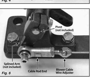
Step 6: Remove the front adjuster nut from the throttle cable adjuster, and insert the throttle cable adjuster into the blower cable bracket. Position the rear adjuster nut so that the blower cable bracket is approximately centered on the threaded part of the throttle cable adjuster. (NOTE: If a Lokar Kickdown Cable is also being installed, you will need to install the kickdown mounting bracket onto the throttle cable adjuster at this time.) Reinstall the front adjuster nut. Fig. 4
