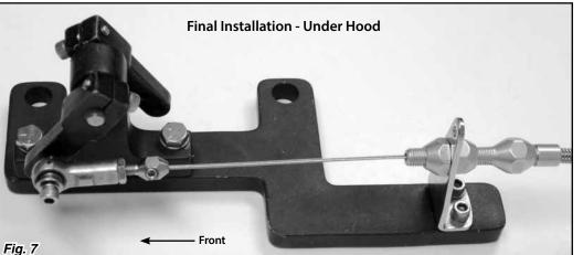
NOTE: Once the Throttle Cable is installed, make sure that the Throttle Pedal is completely floored when the throttle is wide open. If the Throttle Pedal is not completely floored at wide open throttle, you will need to either adjust the pedal itself or install a pedal stop.
