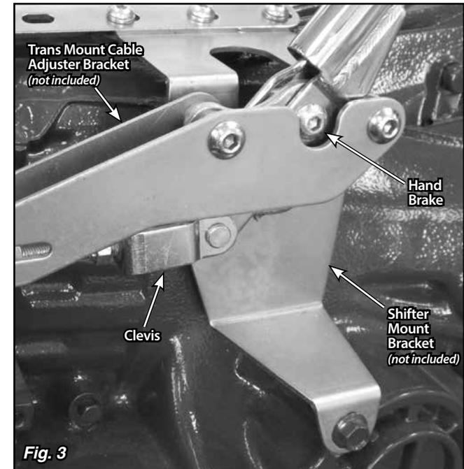
**Step 4:** Follow the instructions for the Transmount Emergency Brake Cable Kit to connect the emergency brake cables. Adjust the Hand Brake so that there is no slack, but make sure that the brakes are not applied when the Hand Brake is released. Generally, you will want the cables adjusted so that three clicks of the Hand Brake will prevent the vehicle from moving (although your braking system may be different). Your completed installation should look like **Fig. 3**.
