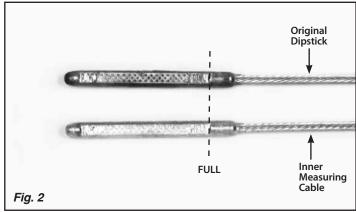
Step 7: Loosen the set screw in the new dipstick handle. Place a drop of clean engine oil or transmission fluid on the upper end of the inner measuring cable, and install the inner measuring cable into the handle. It may be necessary to twist the inner measuring cable (in the direction that tightens the spiral wound strands) in order to get the inner measuring cable into the handle.
